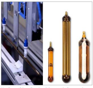
Manufacture of thermally-activated glass ampoules for automatic sprinklers ('e-bulbs')
